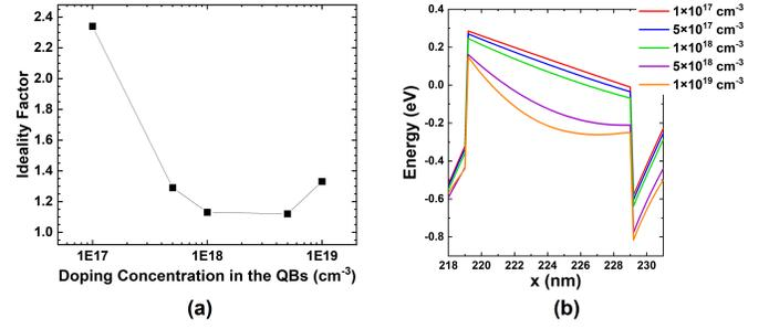
Fig. 3. (a) Ideality factor of the simulated LEDs as a function of doping of the QBs (b) Simulated band diagram of a QB showing doping-induced lowering of barrier potential
