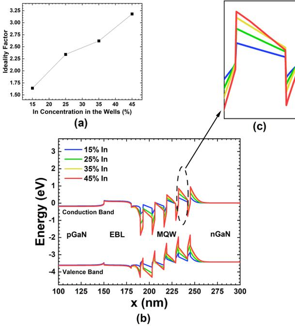
Fig. 2. (a) Ideality factor of the simulated LEDs as a function of Indium incorporation. (b) Simulated band diagram of the LEDs at a forward bias of 3.5 V with (c) an enlarged version of a QB suggesting higher potential barriers for structures with higher In-content
