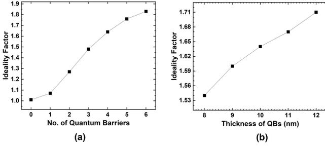
Fig. 1. Ideality factor of the simulated LEDs as a function of (a) No of QBs and (b) thickness of QBs in a 5 QW structure
