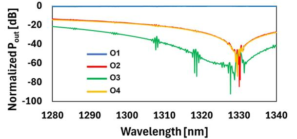
Fig. 6. Normalized transmission characteristics of the 4x4 switch from input-1 to output-1, obtained from Ansys Interconnect simulation.
