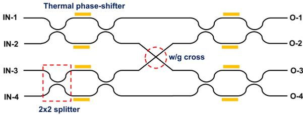
Fig. 4. Schematic diagram of a 4x4 switch.
