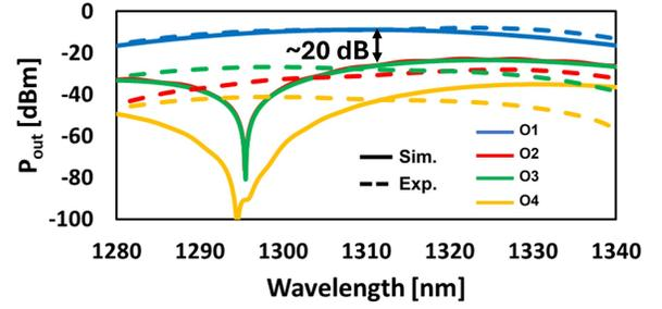
Fig. 5. Transmission characteristics of 4x4 switch from input-1 to output-1. Dashed lines are measured data, solid lines show simulation data.
