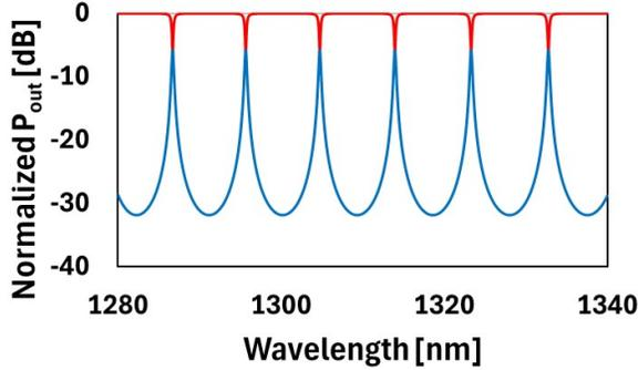
Fig. 3. Normalized transmission characteristics of an add-drop microring resonator obtained from Ansys Interconnect simulation.
