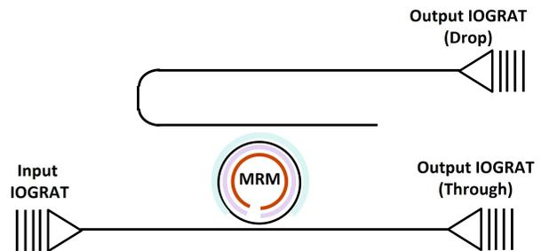
Fig. 1. Schematic diagram of a micro-ring resonator in add-drop configuration.
