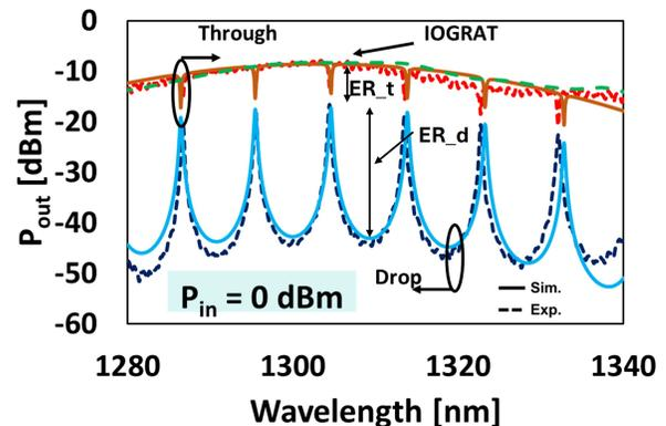
Fig. 2. Transmission characteristics of an add-drop microring resonator for 0 dBm of input power. Solid lines show simulation data from compact model and dotted lines is measured data.
