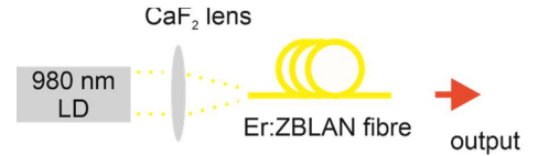
Fig. 1. Experimental setup of an erbium (III) ion doped fluoride glass fiber laser.
