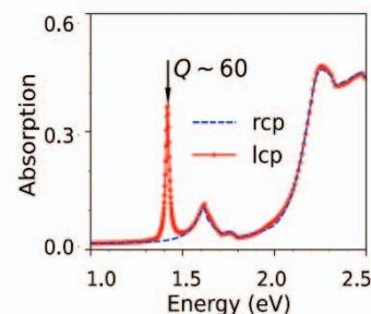
**Fig. 2** Absorption spectra for a metasurface with lattice constant  $a = 500$  nm,  $r_1 = 200$  nm,  $r_2 = 240$  nm,  $r_3 = 160$  nm, at  $\theta = 4^\circ$  for right and left circular polarizations (rcp, lcp), showing a BIC resonance with chiral response.
