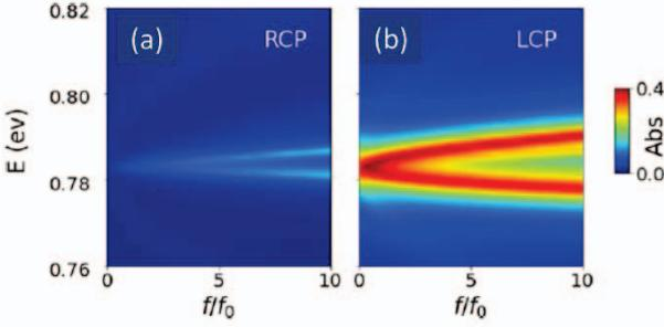
**Fig. 3** Absorption for a metasurface with  $a = 1000$  nm,  $r_1 = 400$  nm,  $r_2 = 480$  nm,  $r_3 = 320$  nm, at  $\theta = 3^\circ$  for rcp (a) and lcp (b). The metasurface contains a resonant medium at the bottom of the nanoholes, in a ring of 50 nm width and 10 nm height, with a linewidth  $\gamma = 0.002$  eV. The absorption map is shown as a function of the oscillator strength of the active medium, in units of  $f_0$  where  $f_0/V = 10^{24}$  m $^{-3}$ .
