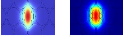
Fig. 2: Electric field distribution of x- and y -polarized modes of the proposed PET fibers.
