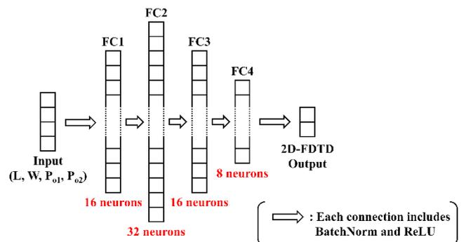
**Fig. 2** Network configuration trained with analyzed data from 2D-FDTD.
