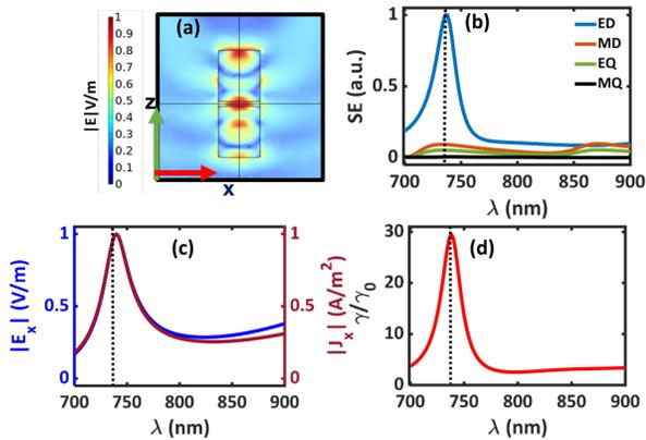
Fig. 2. (a) 2D electric field profile under plane wave excitation in the  $x$ - $z$  plane, showing maximum field confinement near the PVA center. (b) PVA layer's spectral response exhibiting a strong electric dipole (ED) resonance at 738 nm. (c)  $E_x$  and  $J_x$  spectra at the center of the PVA cavity resonant at  $\lambda$ : 738 nm. (d) Relative decay rate spectrum of the SiV center within the PVA cavity.
