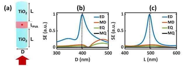
Fig. 1. (a) The schematic of TiO<sub>2</sub> coupled dipole nanoantenna. (b) and (c) The Scattering efficiency (SE) as a function of the diameter (D) and length (L) of the TiO<sub>2</sub> cylinder with maximum SE at D: 400 nm and L: 496 nm respectively.
