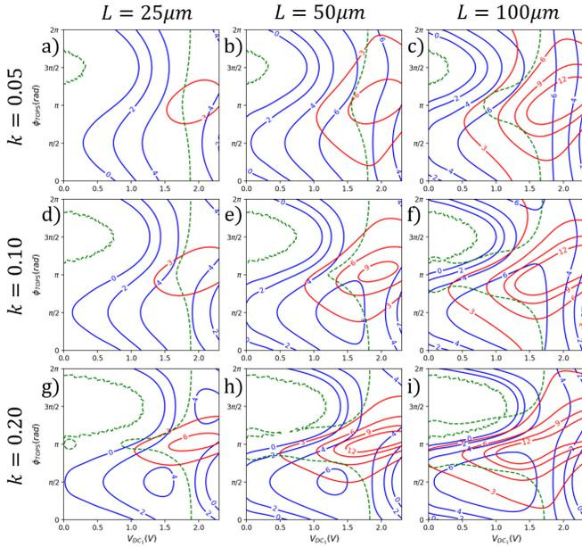
Fig. 2: Contour plots of ER (dB) (red, solid) and OMA (dBm) (blue, solid) as functions of  $V_{DC1}$  and  $\phi_{TOPS}$  for  $k=0.05$ ,  $k=0.10$  and  $k=0.20$  (rows top to bottom respectively) and  $L=25\mu\text{m}$ ,  $L=50\mu\text{m}$  and  $L=100\mu\text{m}$  (columns left to right respectively). The  $\text{CP}=50\%$  contour is indicated by the green dashed lines.
