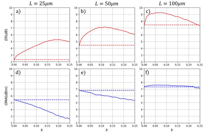
Fig. 3: ER (red, solid) and OMA (blue, solid) of the i-EML with optimised setup conditions ( $V_{DC1}$  and  $\phi_{TOPS}$ ) as a function of  $k$ , with  $L=25\mu\text{m}$  (a, d),  $L=50\mu\text{m}$  (b, e), and  $L=100\mu\text{m}$  (c, f). These results are benchmarked against the ER (red, dashed) and OMA (blue, dashed) of conventional EMLs with the same EAM length and DFB design, equivalent to the i-EML with  $k=0$ .
