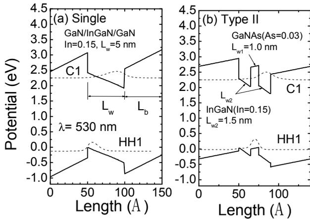
**FIG. 1** potential profiles and the wave functions of the first conduction subband (C1) and the first valence subband (HH1) at zone center for the ground state of (a) conventional InGaN/GaN and (b) type-II InGaN/GaNAs/GaN QW structures.
