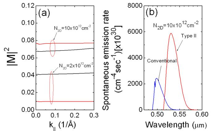
**FIG.2** (a) optical matrix elements and (b) spontaneous emission spectra 530 nm (a) conventional InGaN/GaN and (b) type-II InGaN/GaNAs/GaN QW structures. The SC solutions are obtained at a sheet carrier density of  $N_{2D} = 10 \times 10^{12} \text{ cm}^{-2}$ .
