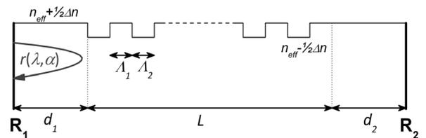
Figure 1. Structural parameters used in the study.
