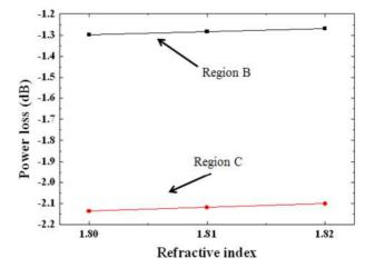
Fig 3. Propagation losses in PLCs as a function of refractive indices of  $SnO_2$  thin films.
