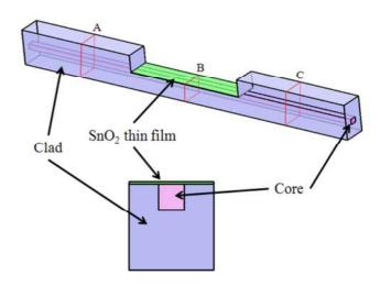
Fig 1. Schematic view of the PLC with SnO<sub>2</sub> thin film.
