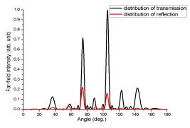
Integration of each distribution curve gives total reflected power (reflectivity R) and transmitted power (transmissivity T). Fig. 4 shows the changing trends of R and T for the four cases.
