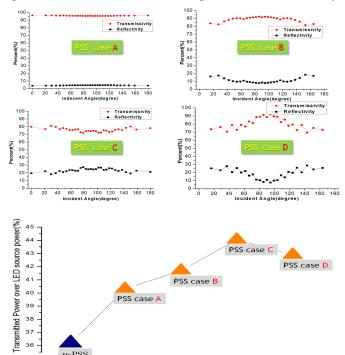
yield a higher LED light power compared with u-PSS LED. Moreover, for PSS cases, as r increases, transmitted light power increases firstly and then drops down after a peak at r=0.5 $\mu$ m. This indicates that micro-structure width (2r) has a strong effect on LED light extraction.
