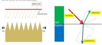
Then in RT simulation, when an incident ray hits PSS interface, *Fresnel* conditions will not be applied. Effective reflection and transmission coefficients are imported from FDTD results. In other words, PSS interface is considered as a
