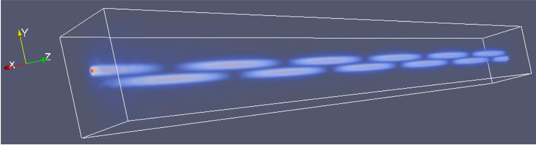
Fig. 2. 3D visualization of BPM simulation of photonic crystal fiber coupler. Computation domain is  $20 \mu\text{m} \times 24 \mu\text{m} \times 2500 \mu\text{m}$ . Scaling along z-direction is 1 : 10.
