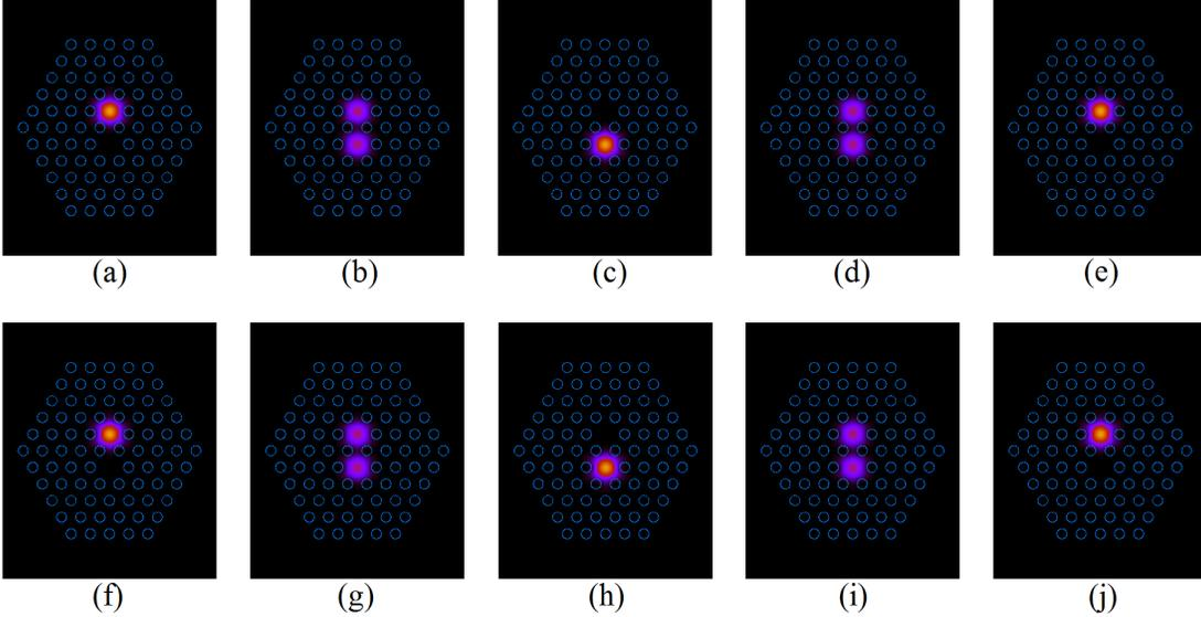
Fig. 3.  $E_x$  power distribution at  $z = 457, 571, 685, 800,$  and  $914 \mu\text{m}$  using (a-e) 15-point scheme with  $\Delta = 0.04 \mu\text{m}$  and (f-j) 28-point scheme with  $\Delta = 0.08 \mu\text{m}$ .
