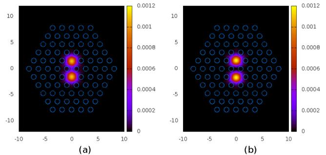
Fig. 1. Simulated  $E_x$  power distribution of (a) even and (b) odd modes.
