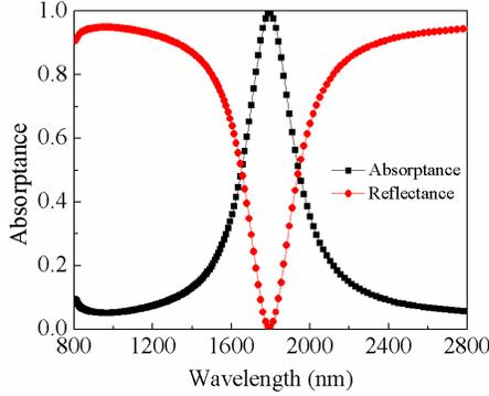
Figure 2. (Color online) Simulated absorption and reflection spectrum of the four-fold rotational symmetrical absorber.
