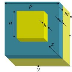
Figure 1. (Color online) Schematic structure of the perfect absorber cell structure. The top layer is square gold particle. The middle and bottom layer are MgF<sub>2</sub> and gold film, respectively.
