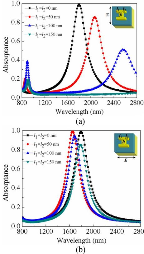
Figure 3. (Color online) The simulated absorption spectra of the two-fold rotational symmetrical absorber with different length of air hole when the polarization of the incident light parallels to  $x$  axis (a) and  $y$  axis (b) , respectively.
