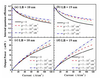
Fig. 2 Simulated IQE and output power for the LEDs with different p-doping concentrations in LB when the thicknesses of the LB are 10 and 19 nm
