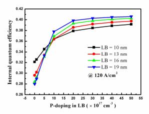
Fig. 3 IQE as a function of p-doping concentration in LB for the LEDs with different LB thicknesses at 120  $A/cm^2$
