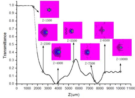
Fig.3. optical power transmittance T of SPPCF and the distribution of propagation mode when R is 0.5 $\mu\text{m}$  and  $\theta = 0^\circ$
