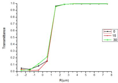
Fig.2. optical power transmittance T of SPPCF vs. residual radius R under different axial rotation angle  $\theta$
