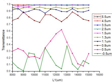
Fig.5. optical power transmittance T of SPPCF calculated vs. the length of flat area with polishing L1 when  $\theta = 0^\circ$
