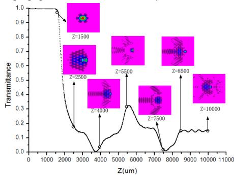
Fig.4. optical power transmittance T of SPPCF and the distribution of propagation mode when R is 0.5 $\mu\text{m}$  and  $\theta = 30^\circ$
