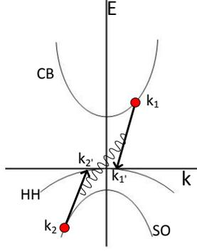
Fig. 2. CHSH Auger recombination showing the first electron,  $k_1$ , recombining with hole,  $k_1$ , passing its energy to the second electron,  $k_2$ , which in turn recombines with hole,  $k_2$ .
