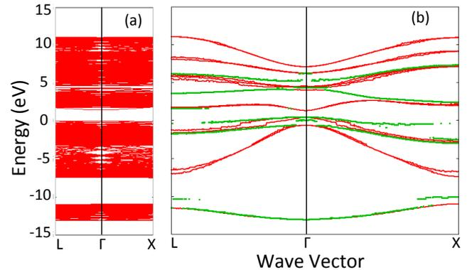
Fig. 1. The (a) folded and (b) unfolded band structure of a 9x9x9 GaAsBi supercell structure at 10% bismuth. Green lines represent defect bands introduced by bismuth.
