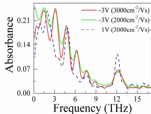
Fig. 2. Plasmon resonances in AlN/GaN HEMTs under different gate voltage.
