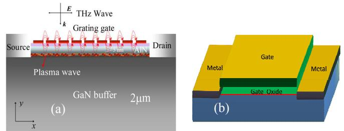
Fig.1. Schematic of device structures: (a) grating-coupled single-channel AlN/GaN HEMT; (b) Graphene device.
