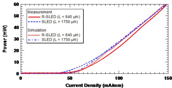
Fig. 1. Measured and simulated front-facet output power of an R-SLED chip with length  $840 \mu\text{m}$  and of a standard SLED chip with length  $1750 \mu\text{m}$  as function of current density. (The current density values are only scaled by the chip length, i. e.  $J = I/L$ . The width of the active area is the same for all devices, and thus, irrelevant for the considerations of this paper.)
