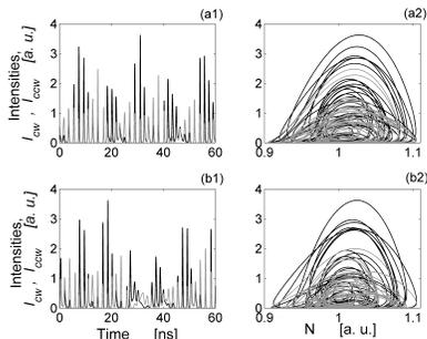
FIG. 2: Panels (a1) and (b1): time series of  $I_{ccw}$  (black) and  $I_{cw}$  (grey). Panels (a2) and (b2): phase portraits. Parameters are:  $\zeta_{OE} = 1.1$  ( $\zeta_{IO} = 0$ ) and  $\tau_{OE} = 2.2$  ns (a),  $\zeta_{IO} = 1.1$  and  $\tau_{IO} = 2.2$  ns (b) with  $\mu = 1.7$ .
