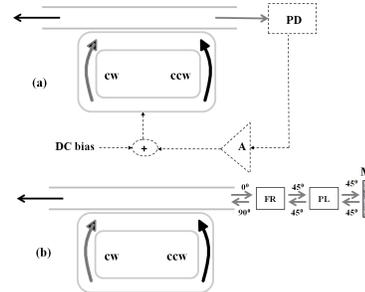
FIG. 1: Schematic diagrams of: (a) SRL-OEF and (b) SRL-IOF. In (a), the solid (dashed) lines indicate the optical (electronic) part. PD—photodetector, A—amplifier, FR—Faraday rotator, PL—polarizer, M—mirror.
