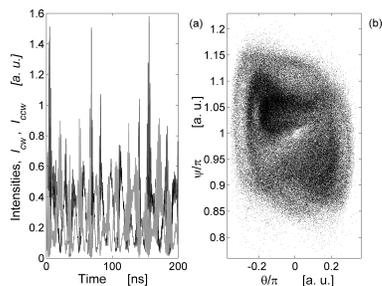
FIG. 3: Time series (a) of  $I_{ccw}$  (black) and  $I_{cw}$  (grey) and the corresponding Poincaré section (b) for  $\zeta_{IO} = 0.8$  and  $\tau_{IO} = 15$  ns.
