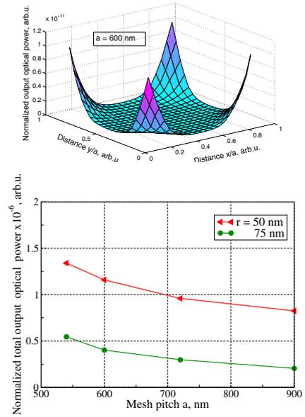
Fig. 2. (a) Spatial distributions of normalized output optical power along mesh window at mesh pitches  $a = 600$  nm; (b) Total normalized output optical power versus mesh pitch  $a$  at different width of the mesh elements.
