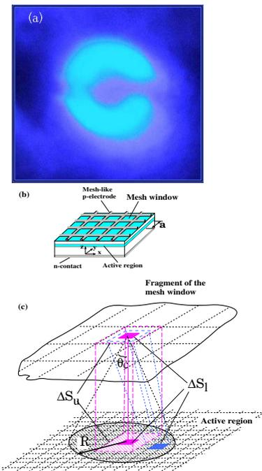
Fig. 1. (a) Emission of blue LED through the windows in the meshed top electrode. (b) Schematic structure of the LED with solid bottom  $n$ - and designed as a mesh top  $p$ -electrodes. (c) A fragment of the LED unit cell in a bi-plane representation. Lower and upper planes correspond to a light-generating layer and output semiconductor-air interface, respectively. NG-cell areas in two planes are different but related to each other.
