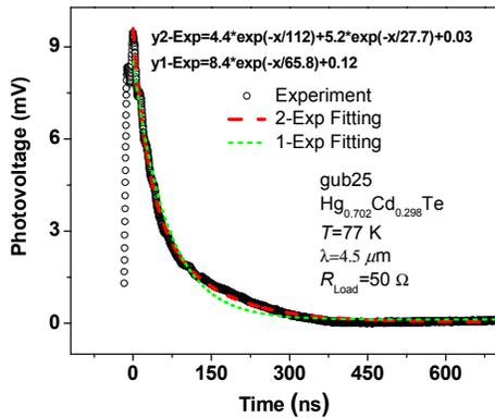
Fig 2. The transient photovoltage curve and the fitting results by using the one-order exponential function and the two-order exponential function.
