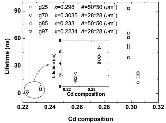
Fig 3. The minority carrier lifetime extracted from the experiment.
