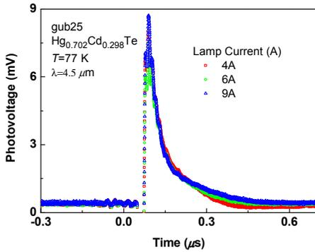
Fig 1 The transient photovoltage of the MCT photodiode with the bias-light intensity and the laser pulses illumination.
