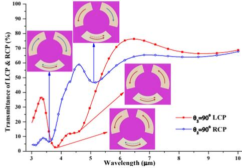
Fig. 2. Normal-incidence LCP and RCP transmittance spectra of the twisted split-ring chiral metamaterials. (Inset figures show the directions of the surface currents on each layer at each resonant frequency, dash lines with arrows for bottom layers and solid lines with arrows for top layers.)
