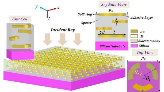
Fig. 1. Schematic of the unit cell for the TSRCMMs structure.
