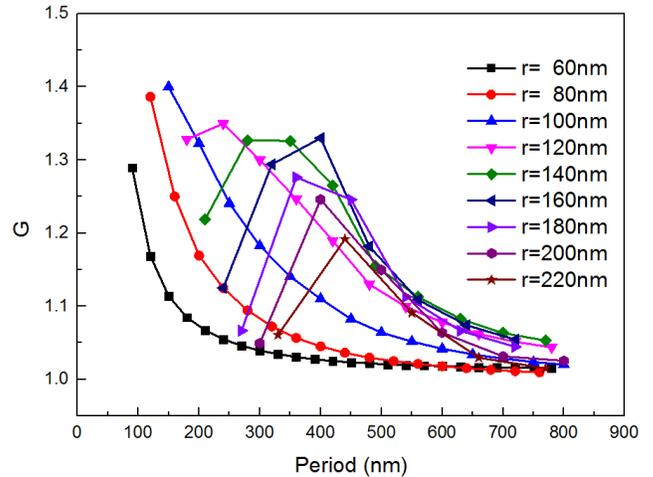
Fig.4 The relation of enhancement factor  $G$  with period at different radii of nanoparticles
