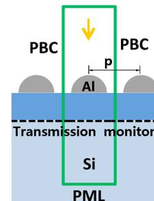
Fig. 1 Schematic of the FDTD simulation model. Al: aluminum nanoparticle; PML: perfectly matched layer; PBC: periodic boundary condition.
