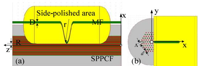
Fig.1. The theoretical coupling model of SPPCF and MF (a) Longitudinal cross-section of optical model; (b) Transverse cross-section of optical model
