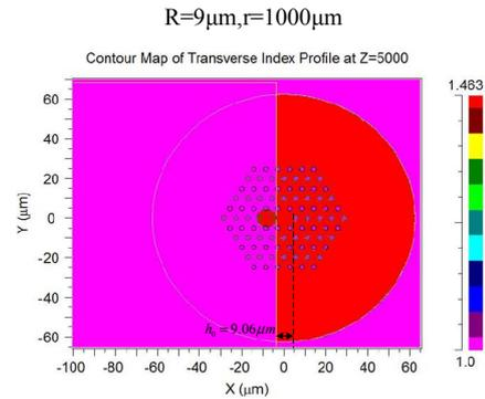
Fig.4 The cross-sectional refractive index distribution of coupling model where  $z=5000\mu\text{m}$
