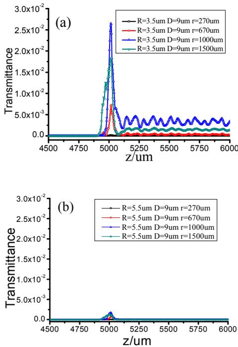
Fig.2 The optical power transmittance  $T$  which is coupled into SPPCF when  $D=9\mu\text{m}$  (a) when  $R=3.5\mu\text{m}$ ; (b) when  $R=5.5\mu\text{m}$
