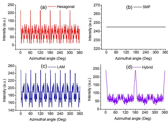
Fig. 3 Simulation results for measured intensity of  $P_1$  at varying azimuthal angle for different fiber. (a) Hexagonal lattice MSF. (b) Single mode fiber. (c) Large area mode MSF. (d) Hybrid lattice MSF. The right column are the cross section of the corresponding fiber.
