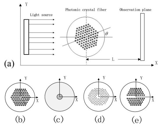
Fig. 1 (a) Schematic diagram of side-imaging technique. Cross sections of sample fibers and definition of azimuthal angles. (b)hexagonal, (c)single mode fiber, (d) larger mode area and(e) hybrid lattice MOF.
