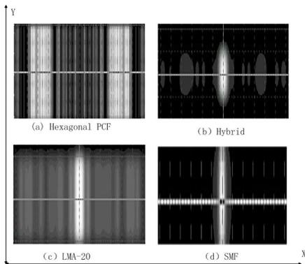
Fig 2. Side image of (a)hexagonal PCF, (b) hybrid PCF, (c) LMA-20 and (d) single mode fiber.
