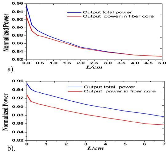
Fig. 3. a).The output normalized power versus  $L$  as  $n_o=1.426$ ; b).The output normalized power versus  $L$  as  $n_o=1.49$
