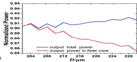
Fig. 4. a).The output normalized power versus  $D$  as  $L=1\text{cm}$ ; b).The output normalized power versus  $D$  as  $L=5\text{cm}$
