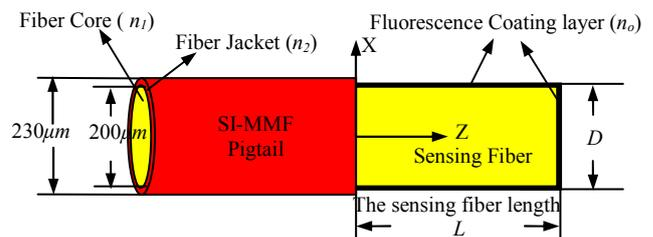
Fig. 1. The model of the fluorescence sensors based on SI-MMFs
