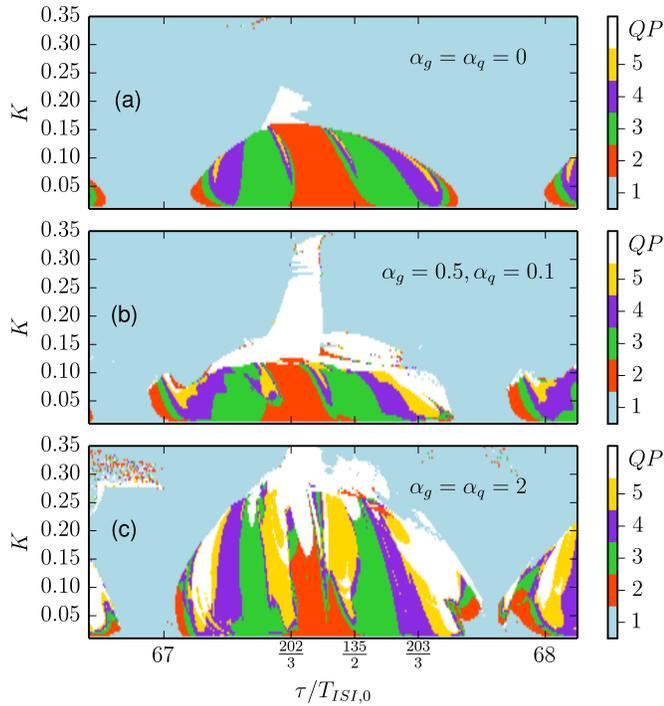
Fig. 1. Bifurcation diagrams as a function of the feedback strength  $K$  and external delay  $\tau$  (in units of the interspike interval of the solitary laser with  $\alpha_g = \alpha_q = 0$ ,  $T_{ISI,0}$ ). Color code: 1-5 indicate the number of pulses in the cavity, regions in white indicate quasiperiodic (QP) ML. Parameters: as in Table I.
