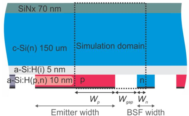
Fig. 1. Schematic representation of the IBC SHJ solar cell with layer thicknesses. To limit the simulation domain we chose a symmetric section of the entire SHJ structure. Note that the varied widths in the simulation,  $W_p$  and  $W_n$ , correspond to half of the entire emitter and BSF stripe width respectively.
