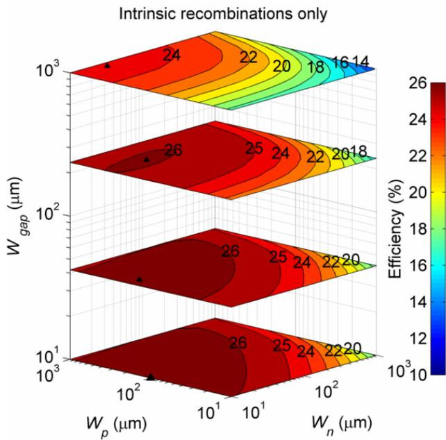
Fig. 2. Efficiency contour plots for wafer with radiative and Auger recombinations only. Contour plots are positioned at  $W_{gap}$  values of 10, 42, 237 and 1000  $\mu\text{m}$ . Black triangles mark the position of the highest efficiency for each  $W_{gap}$  position.
