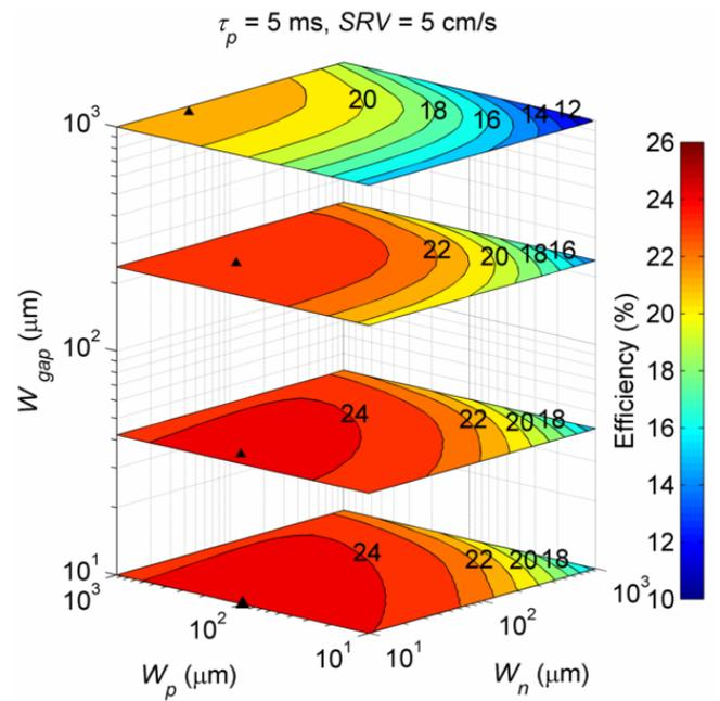
Fig. 3. Efficiency contour plots for wafer with SRH recombinations and non-zero front surface recombination velocity. Contour plots are positioned at same  $W_{gap}$  as Fig. 2. Black triangles mark the position of the highest efficiency for each  $W_{gap}$  position.
