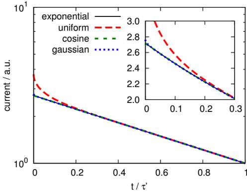
Figure 2. Transient RC-response for different illumination profiles for the case of  $R_E = R_L$ . Uniform illumination causes some deviation from the ideal exponential decay. Illumination with a properly truncated cosine shape reproduces the exponential decay very well. The Gaussian profile fitted to the cosine shape only causes minor deviations. The inset shows a detail with the vertical axis in linear scale.
