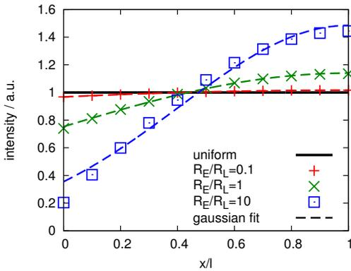
Figure 3. Uniform illumination profile (solid line), truncated cosine illumination profiles (symbols) for different ratios of  $R_E/R_L$ , and the corresponding Gaussian fits (dashed lines).
