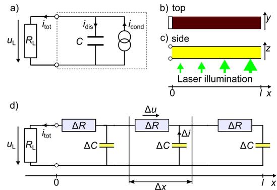
Figure 1. a) The simplified RC-circuit [2]. b) top view and c) side view of the geometry of the photodiode with extended electrodes. The laser profile is graded along the long side of the device. d) Discretized equivalent circuit of a photodiode with extended electrodes [3].
