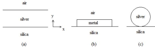
Fig. 1. (a) Schematic of a planar air-silver-silica waveguide. (b) Cross-section of a metal stripe plasmonic waveguide. (c) Cross-section of a silica-substrate-supported silver nanowire.
