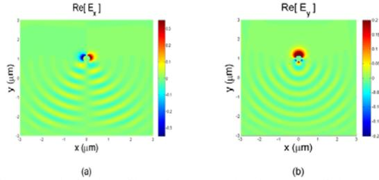
Fig. 4. Mode-field profiles of the second order mode of the structure of Fig. 1(c) when  $\lambda = 500$  nm and  $r = 160$  nm. (a)  $\text{Re}[E_x]$ . (b)  $\text{Re}[E_y]$ .
