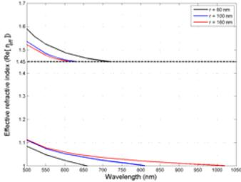
Fig. 5.  $\text{Re}[n_{eff}]$  versus wavelength curves for the first order mode (cutoff at  $n_{eff} = 1.45$ ) and the second order mode (cutoff at  $n_{eff} = 1$ ) of the structure of Fig. 1(c) for three different nanowire radii.
