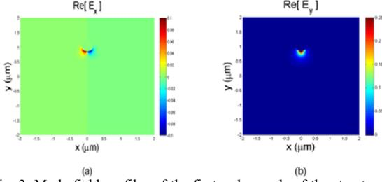
Fig. 3. Mode-field profiles of the first order mode of the structure of Fig. 1(c) when  $\lambda = 500$  nm and  $r = 160$  nm. (a)  $\text{Re}[E_x]$ . (b)  $\text{Re}[E_y]$ .
