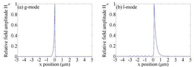
Fig. 2.  $\text{Re}[H_x]$  profiles versus  $y$  position for (a) the pure guided mode and (b) the leaky mode of the planar structure of Fig. 1(a).
