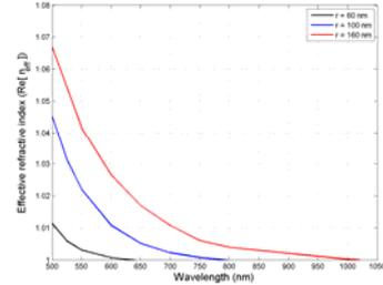
Fig. 7.  $\text{Re}[n_{eff}]$  versus wavelength curves for the second order mode of a nanowire in air for three different nanowire radii.
