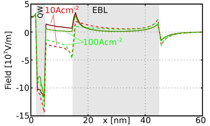
Fig. 3. Electric field in the vicinity of the EBL for graded (dashed) and constant EBL doping (solid) at  $j = 10\text{A/cm}^2$  and  $j = 100\text{A/cm}^2$ .
