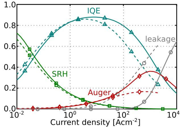
Fig. 4. Relative contribution of SRH (squares), radiative (triangles), and Auger recombination (diamonds) as well as leakage (circles) to the total current for graded (dashed) and constant EBL doping (solid).
