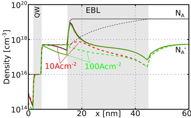
Fig. 2. Acceptor ( $N_A$ ) and ionized acceptor density ( $N_A^-$ ) for graded (dashed) and constant EBL doping (solid) at  $j = 10\text{A/cm}^2$  and  $j = 100\text{A/cm}^2$ .
