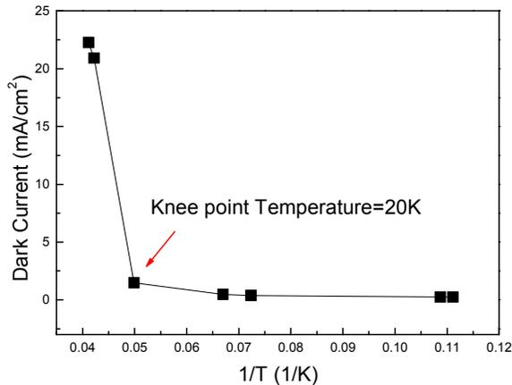
Figure 3. Dependence of dark-current density on the reciprocal of temperature at the bias of 0.2 V.
