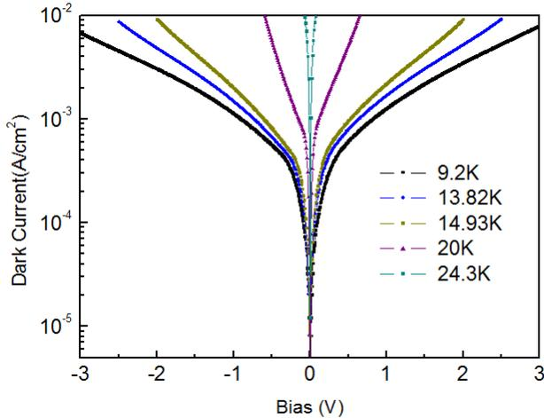
Figure 2. Dark current versus bias of the epitaxial Si:P BIB detector measured in the temperature range from 9.2K to 24.3K and the bias voltage range from -3V to 3V.
