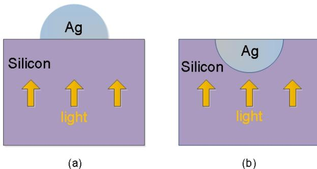
Fig.1 Schematic of the FDTD simulation model. (a) nanoparticle extending into air and (b) nanoparticle extending into silicon.
