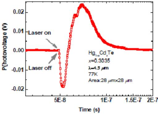
Fig.1 Photoresponse profiles from MCT photodiode illuminated with the Cd composition is 0.3035.
