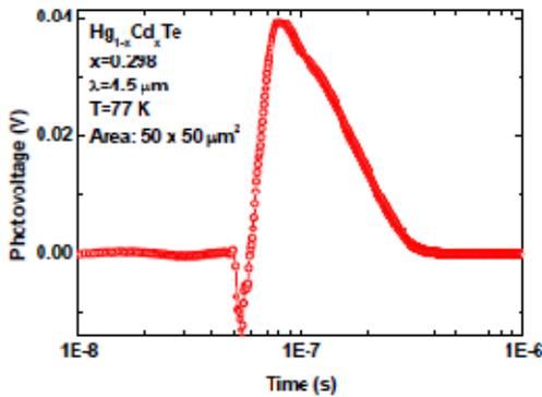
Fig.2 Photoresponse profiles from MCT photodiode illuminated with the Cd composition is 0.298.
