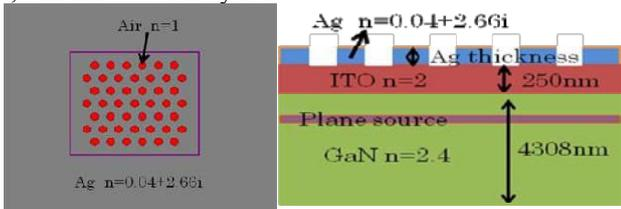
Fig. 2 Schematic illustration of the MPC on ITO surface.
