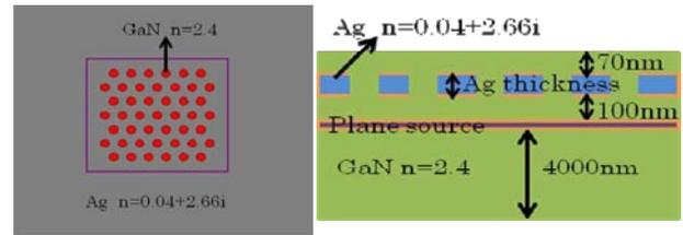
Fig. 4 Schematic illustration of the MPC inside the p-GaN.
