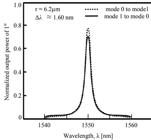
Fig.6. Normalized output power of the converter as function of wavelength  $\lambda$ .
