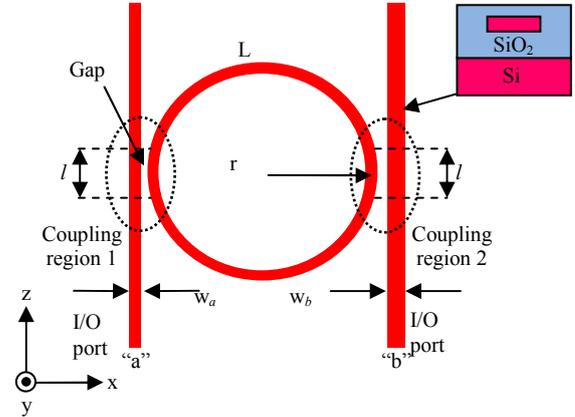
Fig. 1. Proposed ring structure with two different type of coupling region. Here, I/O port widths are different to satisfy the mode accommodation. Device layer is also shown.
