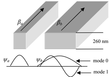
Fig. 2. Straight waveguide assumption in coupling region 2 of the proposed mode converter. Here two waveguides have different width dimension of w<sub>a</sub> and w<sub>b</sub>.
