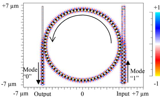
Fig. 5. Electric field ( $E_y$ ) profile of the proposed mode converter. Here, 1<sup>st</sup> mode has been converted to 0<sup>th</sup> mode, which is clearly visible in the profiles.
