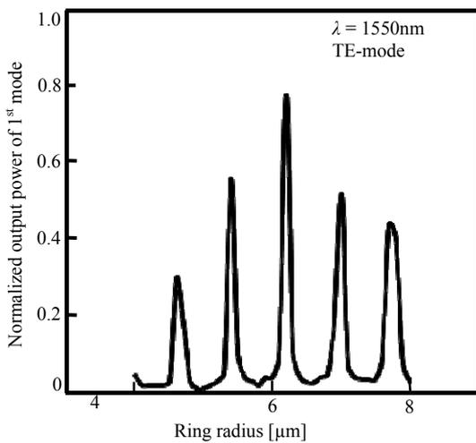
Fig. 4. Effect of ring radius,  $r$  on converted mode power.
