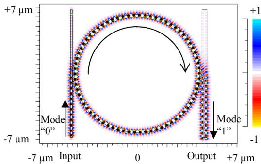
Fig. 3. Electric field ( $E_y$ ) profile of the proposed mode converter. Here, 0<sup>th</sup> mode has been converted to 1<sup>st</sup> mode, which is clearly visible in the profiles.
