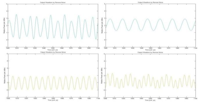
Fig.1(a)~1(d) (left-up for Case F, right-up for Case G, left-bottom for Case K, and right-bottom for Case L): calculated details of output waveform, besides vertical axis is relative output power, dBm, horizontal axis is calculation time, pico-second.
