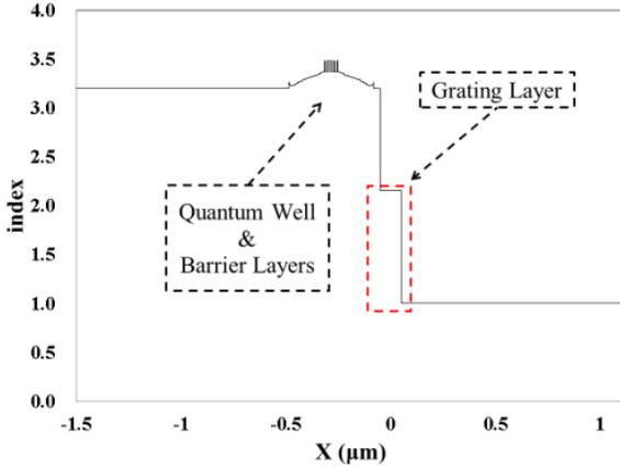
Fig. 2 The index profile of the periodical waveguide in the research.
