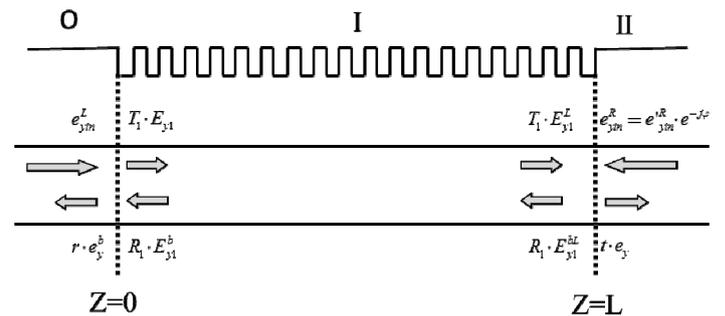
Fig. 1 The basic geometry of the two grating sections.
