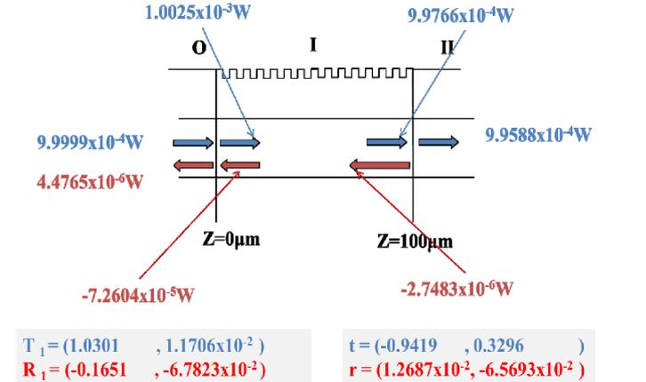
Fig. 4 The calculated power in the non-grating region and the grating region with wavelength of 1315nm.
