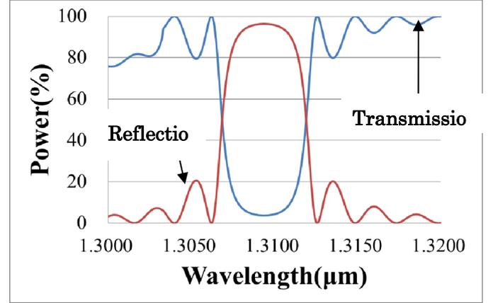
Fig. 3 The transmission and reflection spectra of the periodical waveguide with one grating period of 0.20276985  $\mu\text{m}$  ( $\Lambda$ ).
