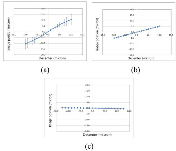
Fig. 3. Image motion as a function of tolerance parameters: (a) decenter of the second surface, (b) decenter of third surface, and (c) decenter of the fifth surface
