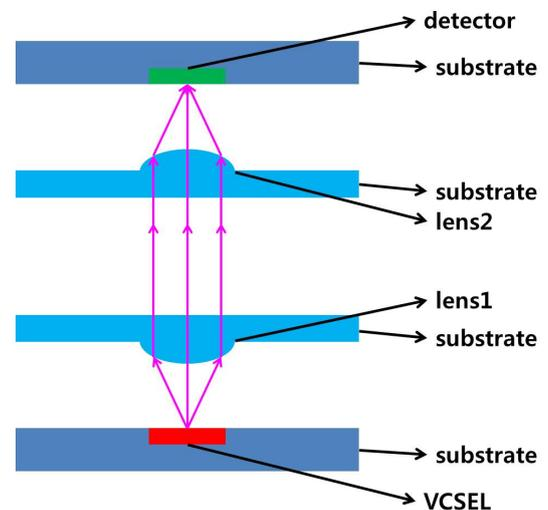
Fig. 1. A free space optical interconnect based on VCSEL, lens, and detector
