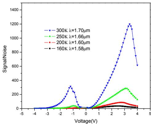
Fig. 4. The SNR as the bias voltage varies from -4V to 4V.
