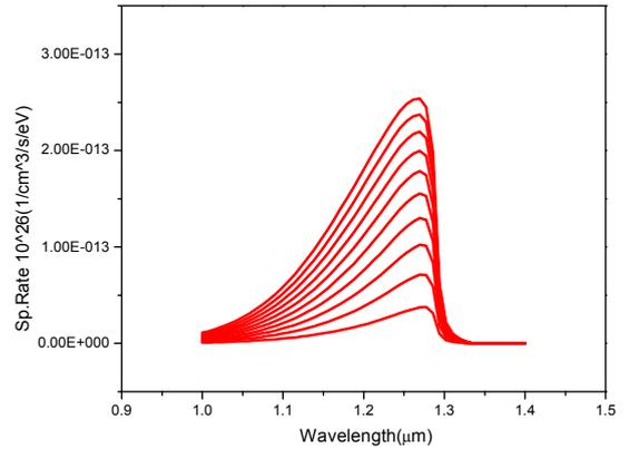
Fig. 5. EL spectrum of InGaAs.
