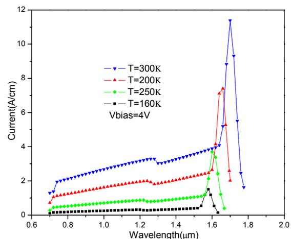
Fig. 1. Photocurrent spectra simulated under different temperature at 4V..
