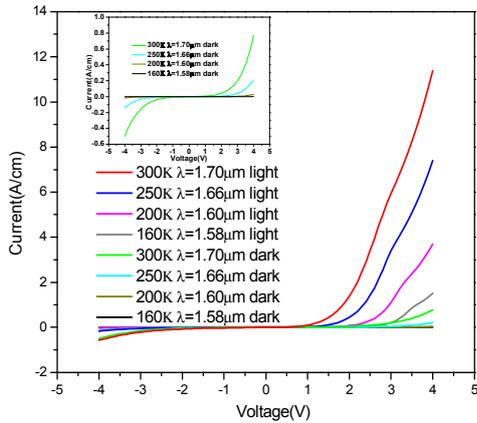
Fig. 3. The I-V characteristics at different incident wavelengths and temperature, insets shows the lower darkcurrent versus the bias.
