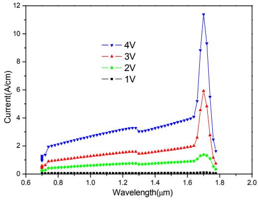
Fig. 2. Photocurrent spectra simulated under different bias at 300K.
