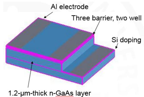
Fig. 1. The simplified 3D view of the device constructed by Lumerical software
