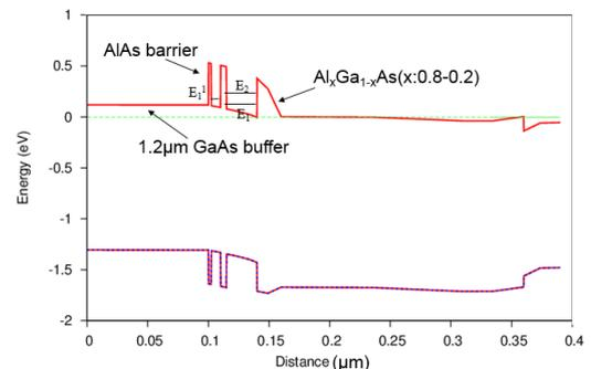
Fig. 2. The band diagram of the device under equilibrium.
