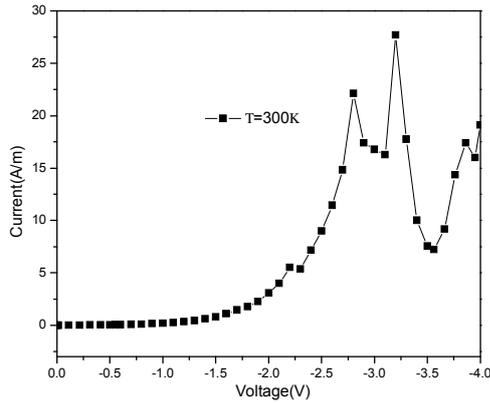
Fig. 3. The I-V characteristics for reverse bias under dark.
