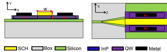
Fig.5 New generation heterogeneous III-V/Si integration based on lateral current injection.
