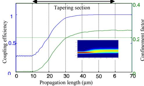
Fig.3 Simulation of adiabatic coupling efficiency.
