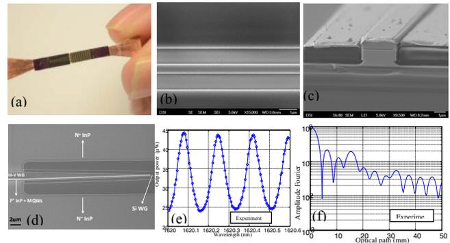
Fig.4 (a-d) fabricated laser device; (e-f) characterization of the FP spectrum response for coupling efficiency and tapering-end reflection.
