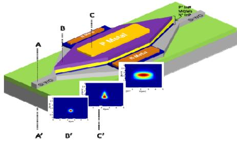
Fig.2 Heterogeneous III-V/Si integration structure and the corresponding mode profile at different position.
