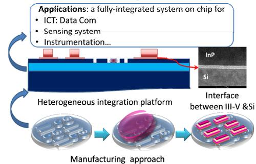
Fig.1 Heterogeneous III-V/Si integration as a platform technology.
