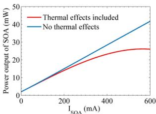
Fig. 3 Optical output power of SOA, with and without thermal effects.
