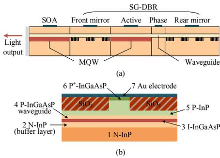
Fig. 1 (a) schematic diagram of the tunable SG-DBR laser integrated with SOA; (b) cross section of the SOA.
