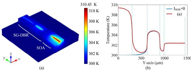
Fig. 2 (a) static temperature distribution when  $I_{SOA}=180 \text{ mA}$ ,  $I_f=I_p=0$ ,  $I_a=100 \text{ mA}$ ,  $I_r=45 \text{ mA}$  and  $P_0=5.2 \text{ mW}$ ; (b) longitudinal static temperature distribution across the center of the laser's active region.
