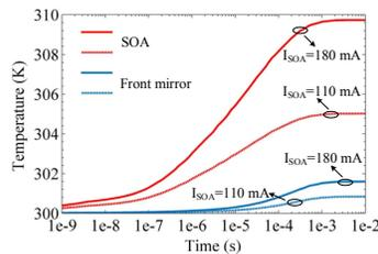
Fig.4 Transient temperature distributions of the SOA and the front mirror section, with  $I_f=I_p=0$ ,  $I_a=100 \text{ mA}$ ,  $I_r=45 \text{ mA}$ ,  $P_0=5.2 \text{ mW}$ .
