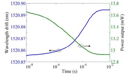
Fig.5 thermal wavelength transients and power output variations when SOA switches on with  $I_{SOA}=180 \text{ mA}$ .
