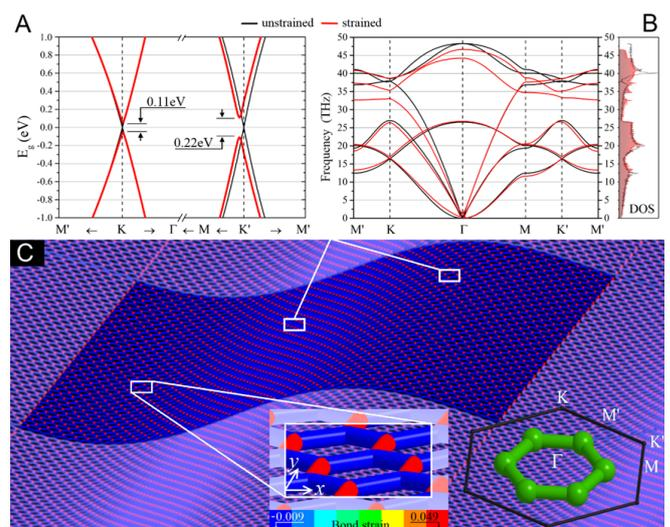
Fig. 1 Graphene sheet under 3.5% compressive strain along x and 3.5% tensile strain along y. Colors in (C) indicate extended (red) or compressed (blue) bonds. The bandstructure (A) exhibits a bandgap of 0.22eV at the  $K'$  point of the Brillouin zone.[3]
