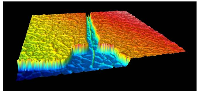
Fig. 3. AFM of a Graphene sheet between two metal contacts with a separation of 1 $\mu$ m. The Graphene is subjected to compressive strain resulting in the formation of a stable nm-sized ripple in the middle of the gap.
