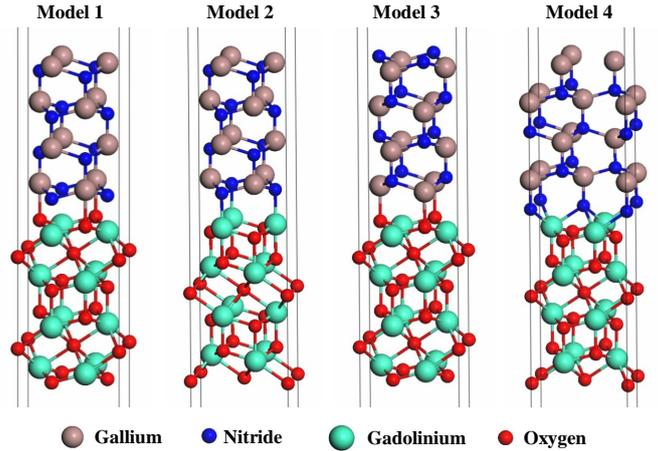
FIG. 1. Atomistic representations of the four GaN/Gd<sub>2</sub>O<sub>3</sub> interface models with a  $1 \times \sqrt{3}$  basal dimension in the hexagonal lattice structure. Models 1 and 2 have Ga-polar GaN surfaces, while models 3 and 4 have N-polar GaN surfaces. The atoms are represented by spheres: Ga (brown), N (blue), Gd (green), and O (red). (For interpretation of the references to color in this figure legend, the reader is referred to the web version of this article).
