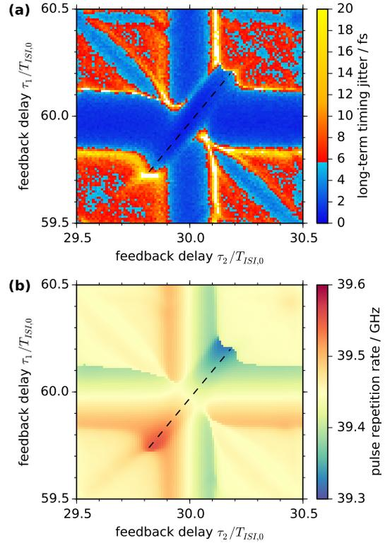
Fig. 3. (a) Long-term timing jitter for the single PMLL with a dual optical feedback scheme. The color code shows the timing jitter in dependence of the two feedback delays  $\tau_1, \tau_2$ . (b) Pulse repetition rate in dependence of the two feedback delays. The dashed line in both panels denotes a parameter range for which strong suppression of the timing jitter along with a tuning of the pulse repetition rate over several hundred MHz is possible.  $K_1^{fb} = K_2^{fb} = 0.05$ .
