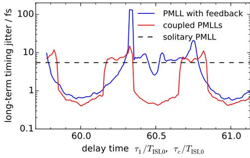
Fig. 2. Long-term timing jitter in dependence on the optical delay times  $\tau_1$  for the PMLL with single optical feedback (blue), and on the coupling delay time  $\tau_c$  for two coupled PMLLs. The delay times are given in units of the solitary PMLL inter-spike interval time  $T_{ISI}$ . The dashed line denotes the timing jitter of the solitary PMLL.  $K_1^{fb} = 0.1$ ,  $K_2^{fb} = 0$ ,  $K_c = 0.1$ .
