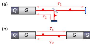
Fig. 1. Sketch of the passively mode-locked laser (PMLL) control schemes: (a) PMLL with delayed optical feedback. (b) Delayed coupling of two PMLLs.  $G$  and  $Q$  denote gain and absorber sections, respectively.
