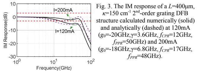
Fig. 3. The IM response of a  $L=400\mu\text{m}$ ,  $\kappa=150\text{cm}^{-1}$  2<sup>nd</sup>-order grating DFB structure calculated numerically (solid) and analytically (dashed) at 120mA ( $g_0=-20\text{GHz}$ ,  $\gamma=3.6\text{GHz}$ ,  $f_{CPR}=12\text{GHz}$ ,  $f_{PPR}=50\text{GHz}$ ) and 200mA ( $g_0=-18\text{GHz}$ ,  $\gamma=6.8\text{GHz}$ ,  $f_{CPR}=17\text{GHz}$ ,  $f_{PPR}=48\text{GHz}$ ).
