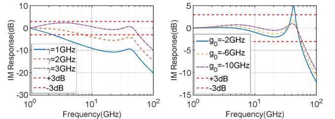
Fig. 2. The impact of parameters  $\gamma$  and  $|g_0|$  on the IM response. Left: increase  $\gamma$  while keeping  $g_0=-10\text{GHz}$ ,  $f_{CPR}=10\text{GHz}$ ,  $f_{PPR}=40\text{GHz}$ ; Right: increase  $|g_0|$  while keeping  $\gamma=6\text{GHz}$ ,  $f_{CPR}=10\text{GHz}$ ,  $f_{PPR}=40\text{GHz}$ .
