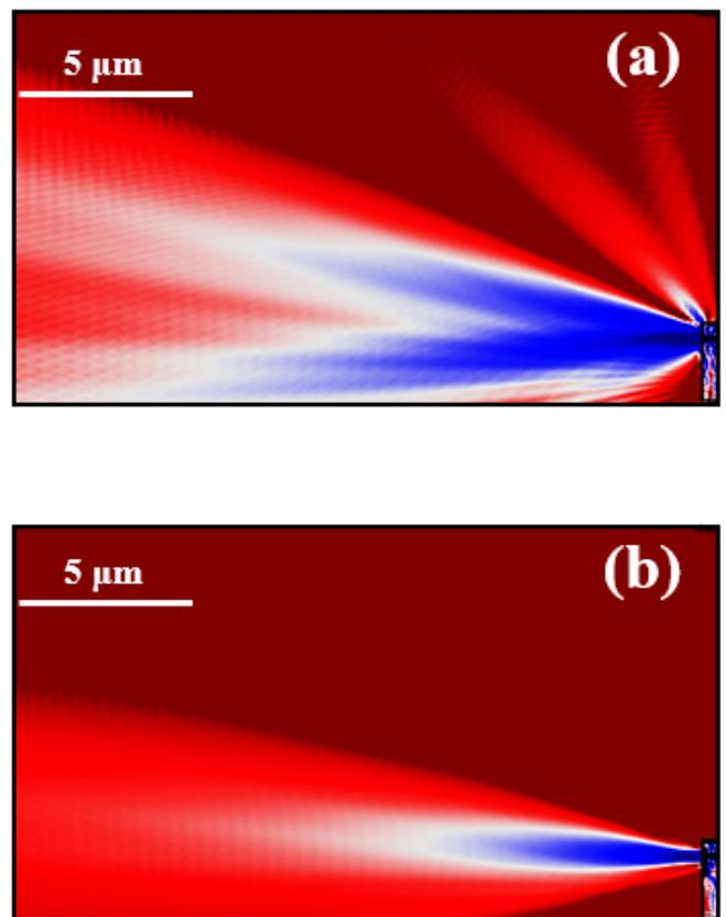
Fig. 1. (a) 2D calculation of the intensity distribution of an original unpatterned GaN-based design. (b) 2D calculation of the intensity distribution of a small-divergence GaN-based design.
