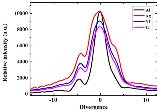
Fig. 2. Four types of covered metal materials corresponding to the simulated far-field intensity distribution of the GaN-based device with patterned metallic coating.
