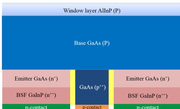
Fig. 1: Simulation model of all-back-contact GaAs solar cells
