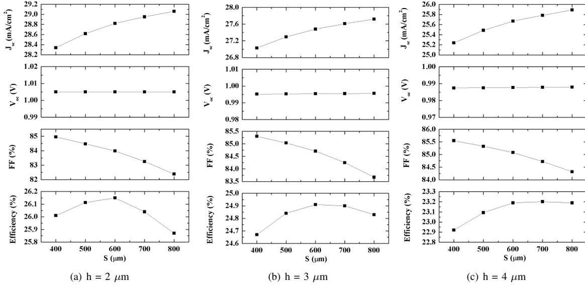
Fig. 2: Characteristics of all-back-contact GaAs solar cells
